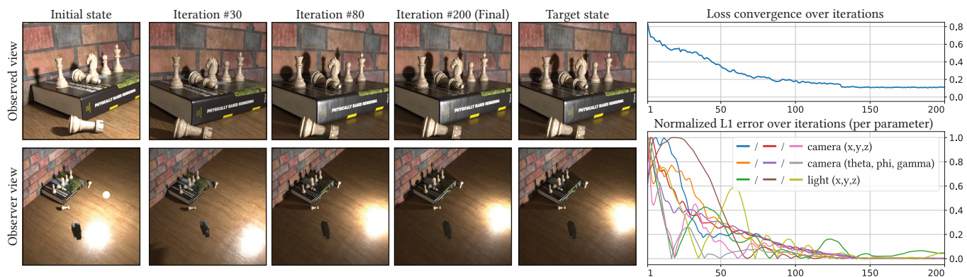
Fig. 15. 6D camera pose and light position estimation in a scene with complex light transport involving soft shadows and glossy interreflections. Top : Camera view at different steps during optimization. Bottom : Visualization of the scene from the top at the same steps (camera shown as an actual object). Right : Convergence of the loss and error plots of the 9 parameters that are jointly optimized. The supplemental video shows an animated version of this result.
